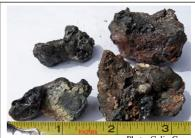
Photo Colin Gross Pieces of clinker, which will form a solid layer over the grate and stifle the fire if not raked out.
